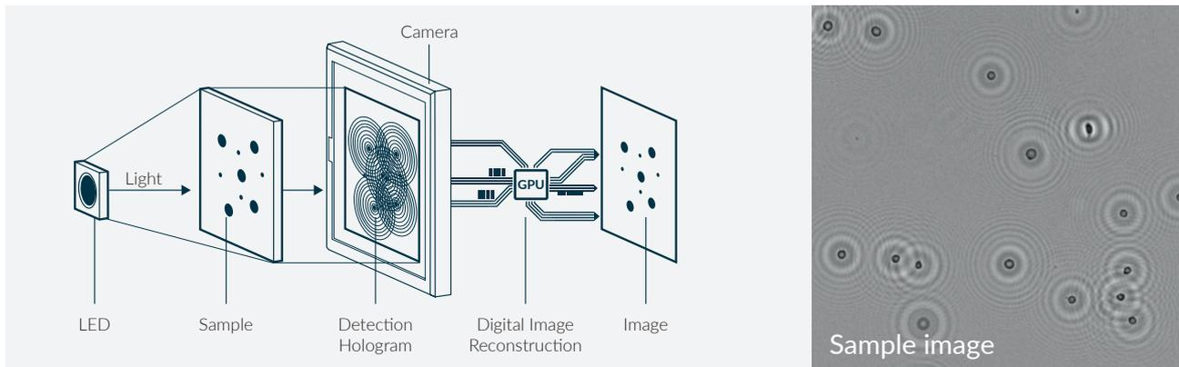
Digital holographic microscopy (DHM) is a state-of-the-art quantitative phase imaging technique that allows automated label-free analysis of cell counts and viability. In DHM, the sample is illuminated with light. As light passes through the sample, some of it
