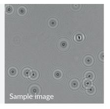
Digital holographic microscopy (DHM) is a state-of-the-art quantitative phase imaging technique that allows automated label-free analysis of cell counts and viability. In DHM, the sample is illuminated with light. As light passes through the sample, some of it
