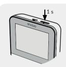
Turn on the device by pressing the button on top for 1 s. The screen will turn on after 15 s. The device goes into stand-by if not used. Tap on the screen to activate the display.
