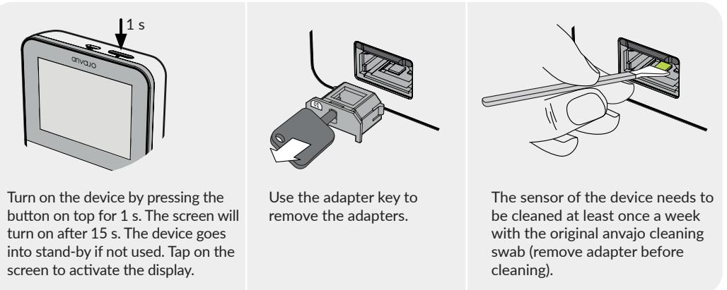
Turn on the device by pressing the button on top for 1 s. The screen will turn on after 15 s. The device goes into stand-by if not used. Tap on the screen to activate the display.
