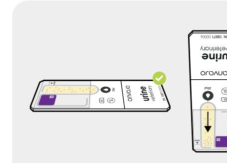
11. Start the measurement on the device **immediately** after filling the sample carrier to minimize errors caused by evaporation of the sample and / or gravity sedimentation of high-density elements.
