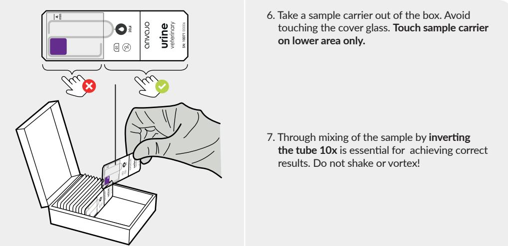
6. Take a sample carrier out of the box. Avoid touching the cover glass. **Touch sample carrier on lower area only.**
