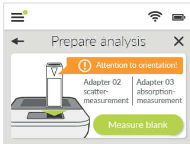
Figure 11: Insert cuvette in the right orientation before measuring blank.
